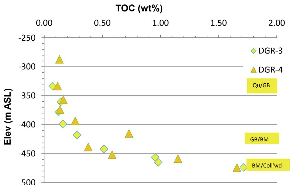
**Figure 4.13: TR-08-29, Laboratory Organic Geochemistry Testing of DGR-3 and DGR-4 Core**
