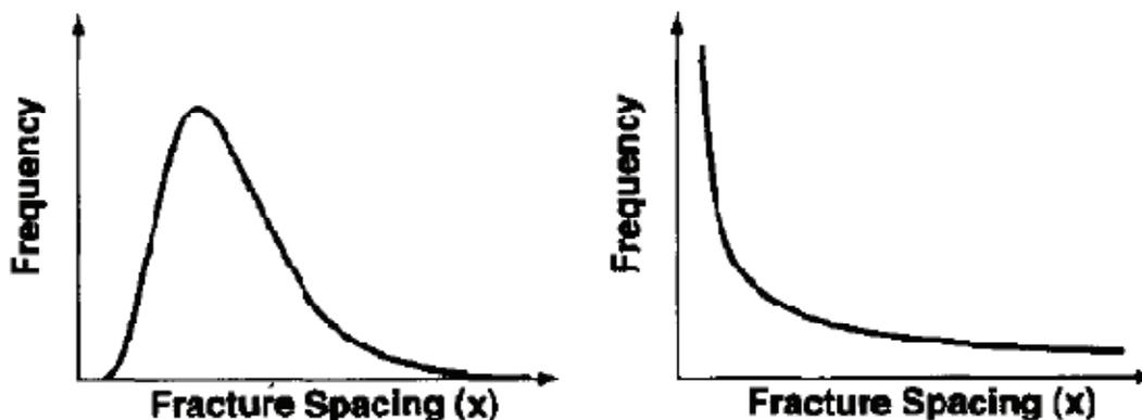
Notes: From Gross and Engelder (1995). Left: Log-normal distribution of vertical joints that may be characteristic of the seal rocks at the DGR site. Right: Power-law distribution of fractures with a variety of orientations that may be characteristic of the upper 200 m of rock at the Bruce nuclear site.
