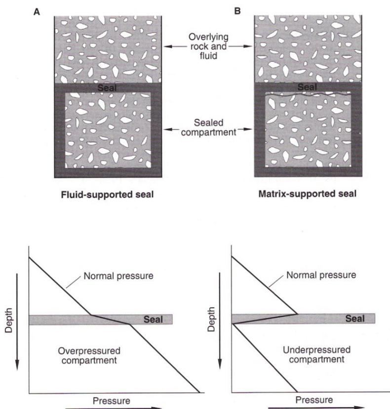
Notes: (A) Pressure/depth gradient from normal pressure to overpressure across the hydraulic seal surrounding the overpressured rock section. (B) Pressure/depth gradient from normal to underpressured rock across the hydraulic seal surrounding the underpressured rock section (after Hunt 1996).
