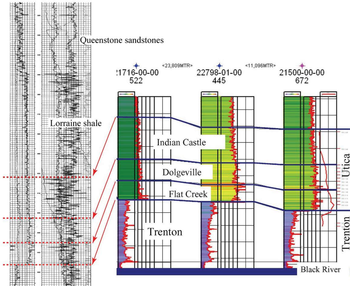
Notes: Adapted from Nyahay et al. (2007). Three color logs on the right are gamma ray logs. The log on the left is the raster log for 22798-01-00 showing both a gamma ray (left) and density track (solid line on right).
