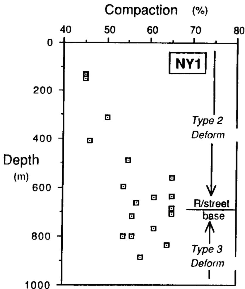
Notes: To estimate overburden compaction the chlorite strain had to be normalized for the type of layer-parallel shortening developed during Alleghanian shortening. Type 2 layer-parallel shortening deformation is uniaxial parallel to bedding (type u) whereas Type 3 layer-parallel shortening deformation is volume constant strain (type v). Adapted from Oertel et al. (1989).
