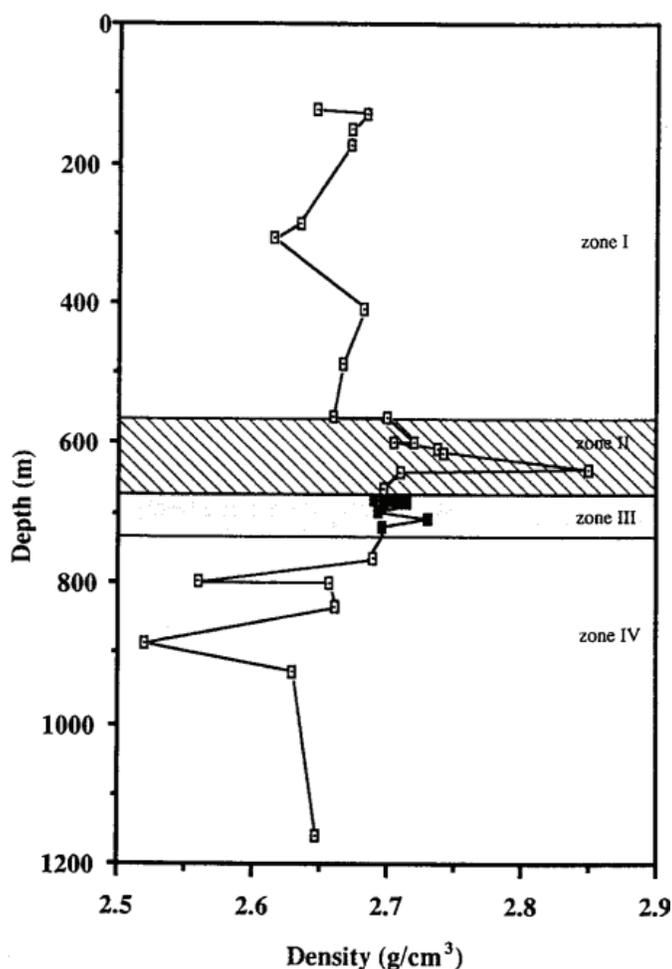
Notes: Shale densities (as measured in a heavy liquid column) peak in and above the transition zone, but decrease in the lower stress regime, indicating undercompaction of the deeper seated rocks. These data are consistent with strain measurements mentioned earlier in the text. Adapted from Albrecht (1992).
