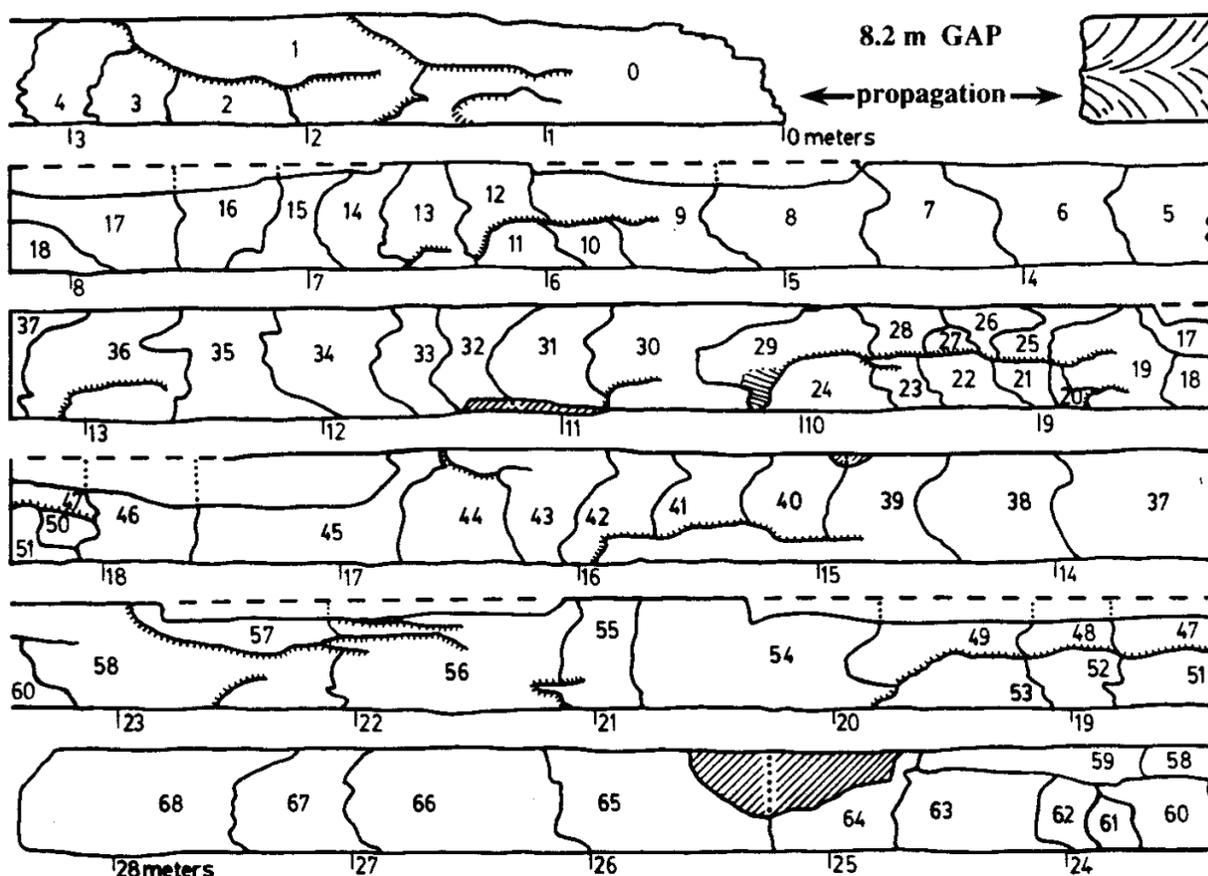
Notes: Joint propagated in discrete increments which are numbered in order of development as determined by morphological criteria, adapted from Lacazette and Engelder (1992).
