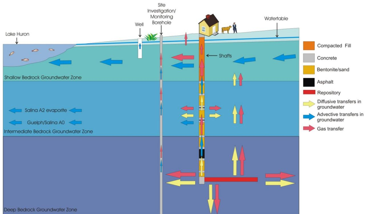
Figure 4-1: Open Borehole Scenario
