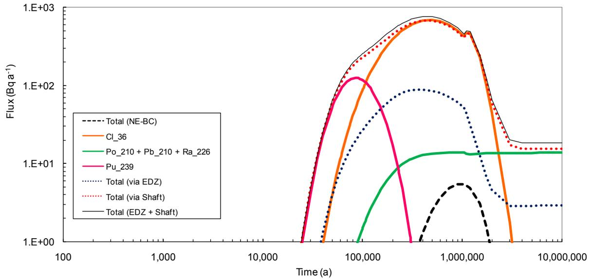
**Figure 3-6: Calculated Fluxes of Contaminants in Groundwater through the Shaft for the Severe Shaft Seal Failure Scenario (Degradation of Upper Shaft Only), Compared with Results for the Normal Evolution Scenario**
