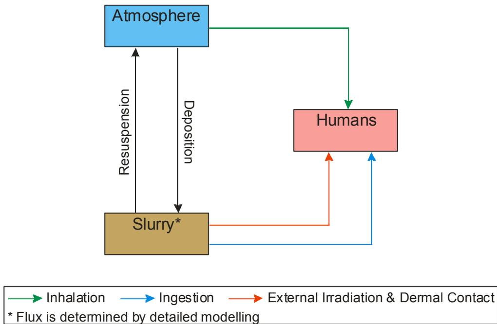
**Figure 2-3: Human Intrusion Scenario: Conceptual Model for Exposure of the Drill Crew During the Slurry Release**
