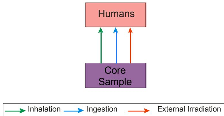
**Figure 2-6: Human Intrusion Scenario: Conceptual Model for Core Retrieval**
