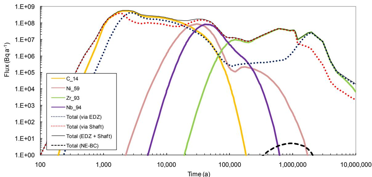
**Figure 3-5: Calculated Fluxes of Contaminants in Groundwater through the Shaft for the Severe Shaft Seal Failure Scenario (Degradation of Entire Shaft), Compared with Results for the Normal Evolution Scenario**
