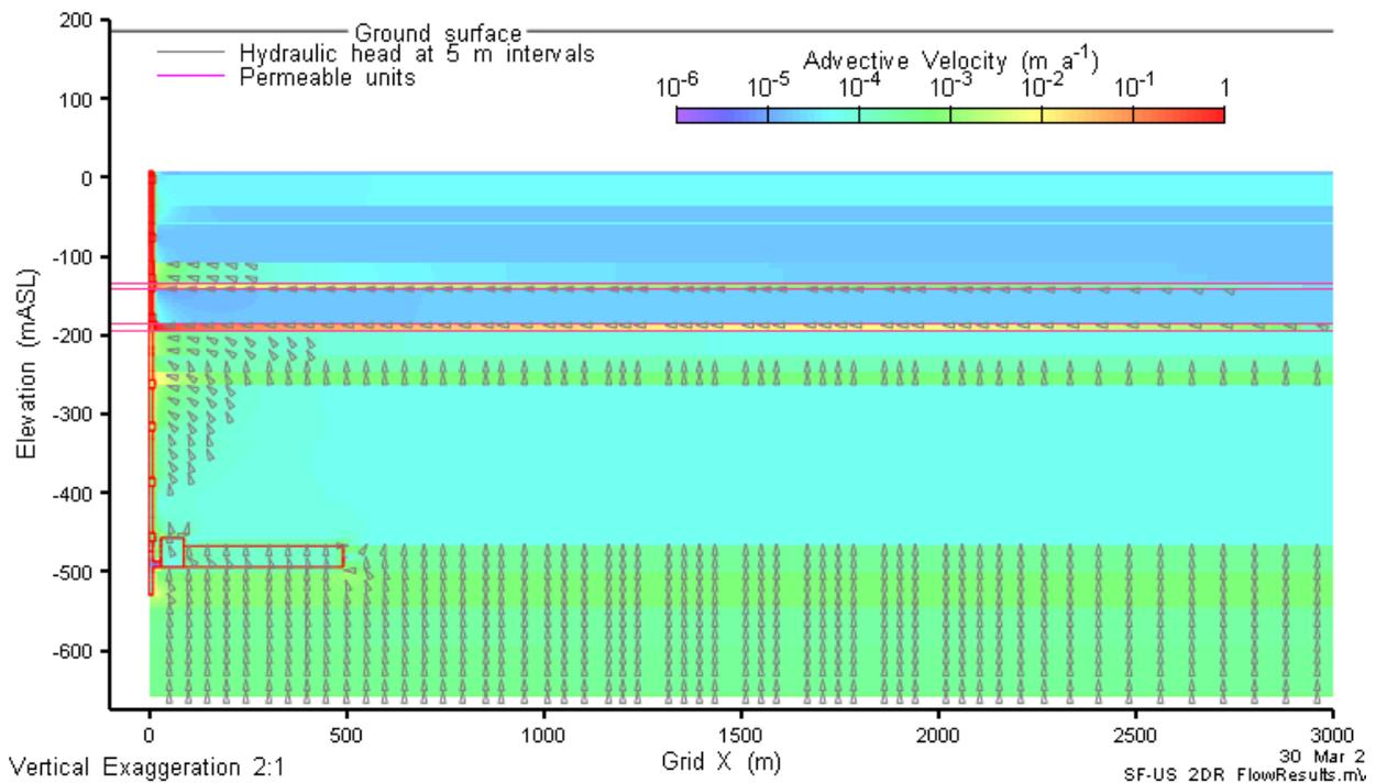
**Figure 3-4: Advective Velocities for the Severe Shaft Seal Failure Scenario SF-US-F2 Case**
