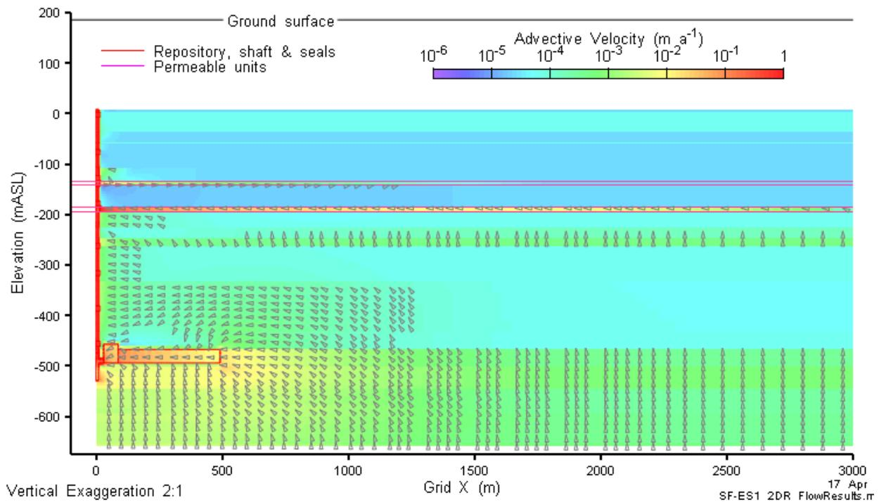
**Figure 3-3: Advective Velocities for the Severe Shaft Seal Failure Scenario SF-ES1-F2 Case**
