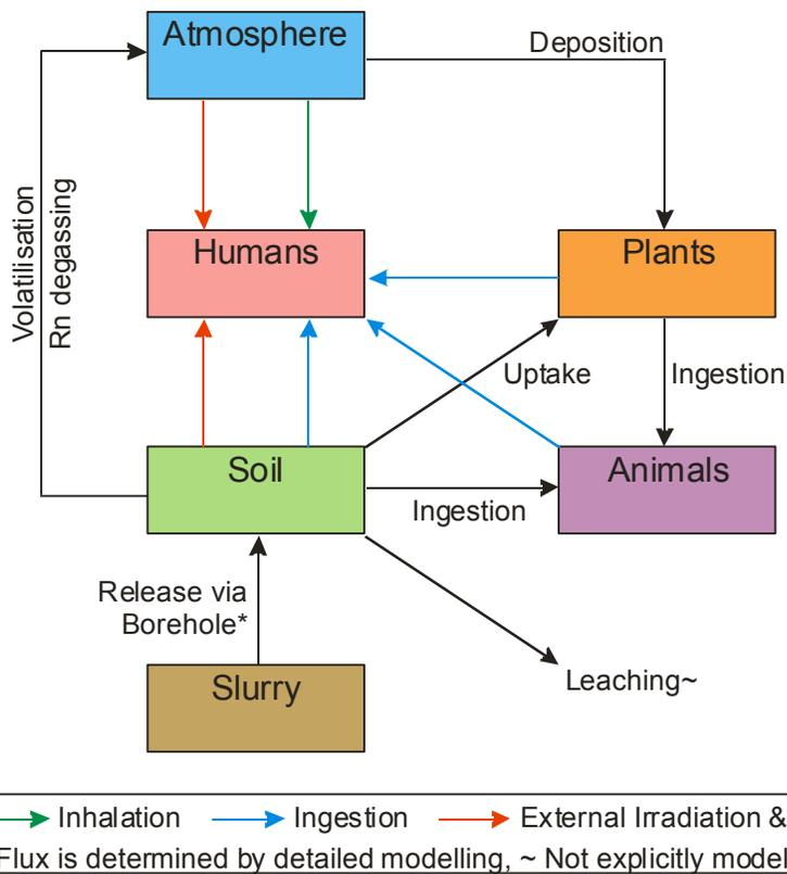
**Figure 2-4: Human Intrusion Scenario: Conceptual Model for Exposure of the Site Resident to Soil Contaminated by Slurry**
