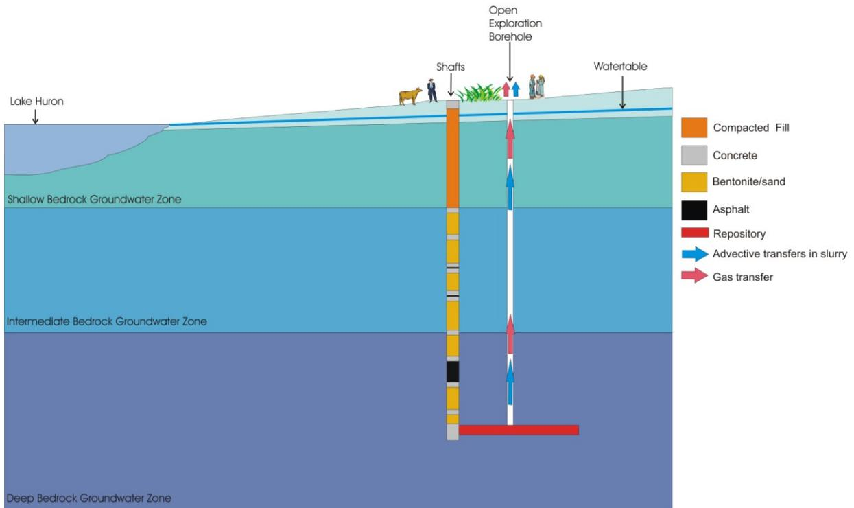
**Figure 2-1: Human Intrusion: Schematic Representation of Short-term Gas and Slurry Releases**
