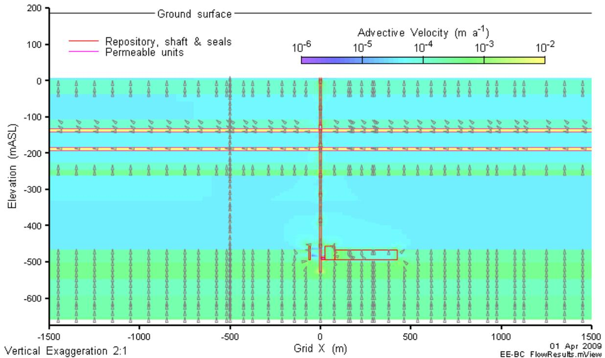
**Figure 5-2: Advective Velocities for the Extreme Earthquake Scenario EE-BC-F3 Case**
