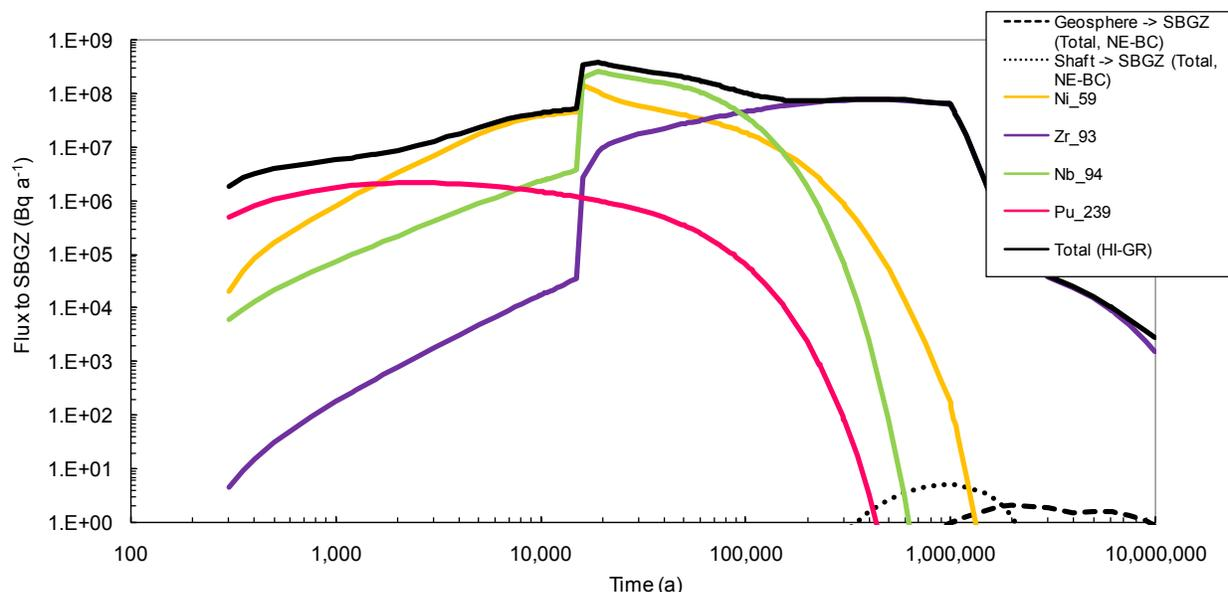
**Figure 2-14: Flux of Contaminants Released via an Intrusion Borehole Drilled 300 years after Repository Closure**
