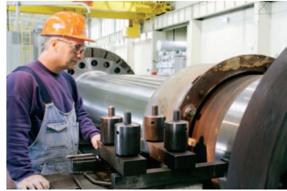
OPG Mechanical Technician , Doug Douma, cleaning a turbine shaft as part of refurbishing generation Unit 14 at the Beck 2 hydroelectric station in Niagara Falls. The refurbishment is part of a major long-term upgrade program of all 16 units at the station, begun in 1996, and scheduled for completion in 2005. When complete, the program will have added 194 MW of capacity to the station.
