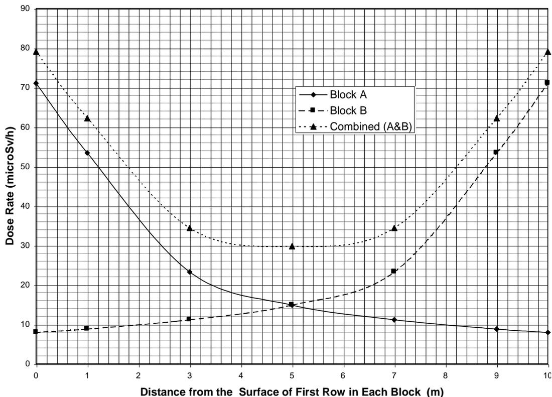
Figure 13: Calculated Dose Rates Inside a DSC Storage Building – North-South Corridor
