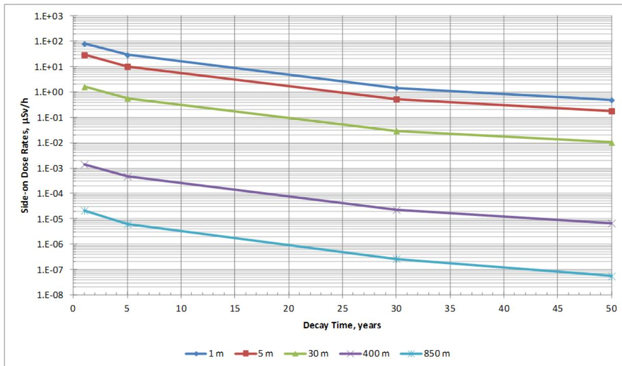
**Figure 6: Estimated Dose Rates from a DSM Containing Retube Components from Unit 3/4**
