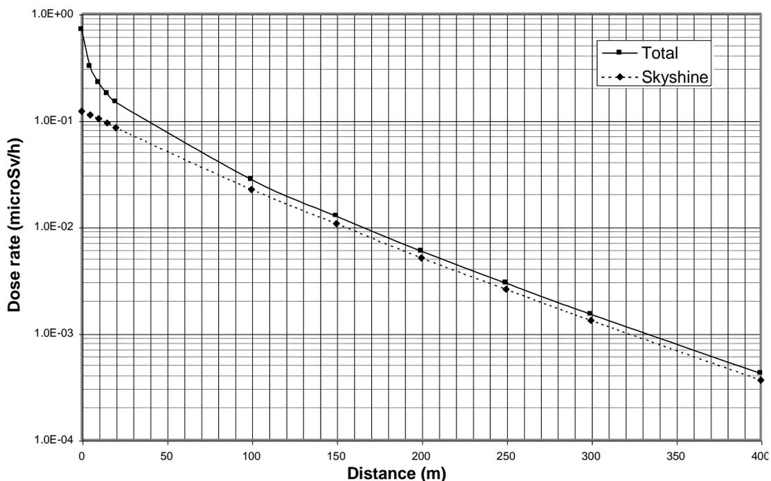
**Figure 15: Calculated Dose Rates from Phase II DSC Storage Buildings – North/South Walls**
