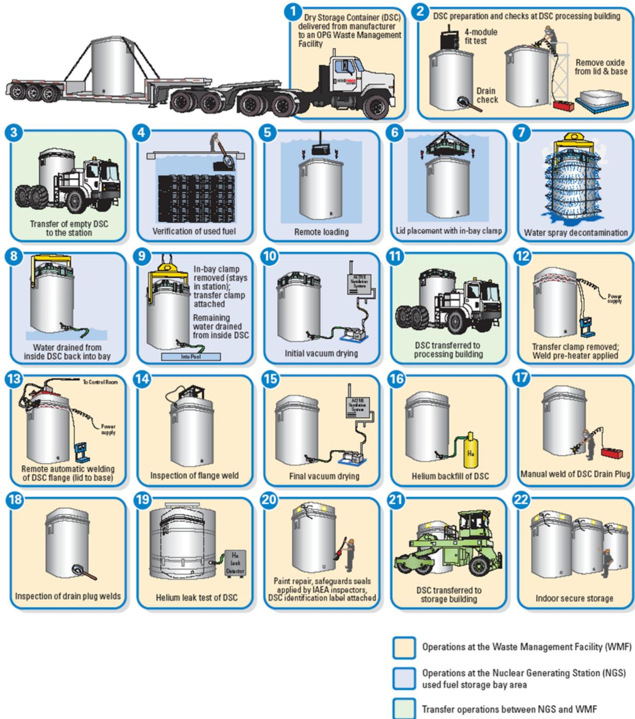
Figure 8: Used Fuel Dry Storage Process
