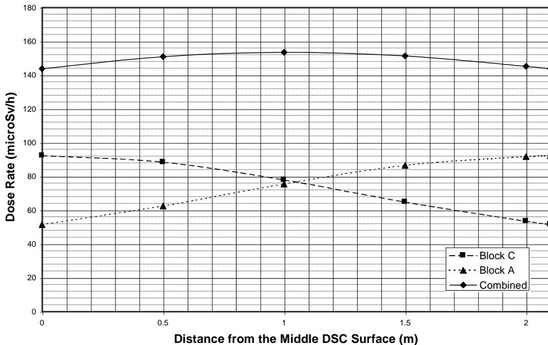
**Figure 12: Calculated Dose Rates Inside a DSC Storage Building – East-West Corridor**
