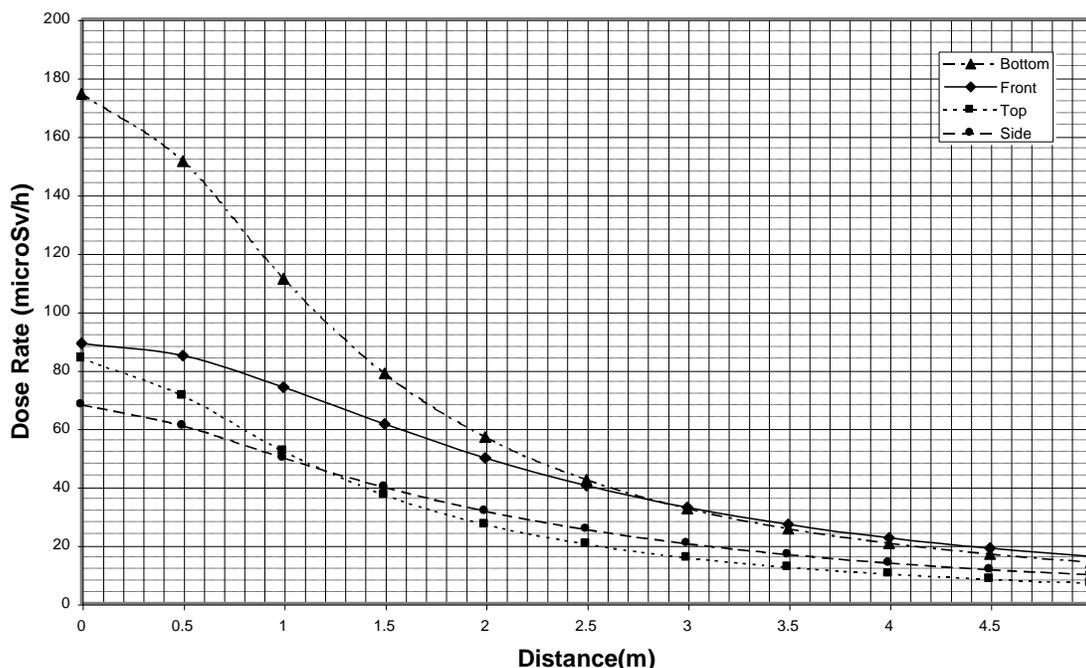
**Figure 11: Calculated Dose Rates from a DSC Containing 10-Year-Cooled Used Fuel**
