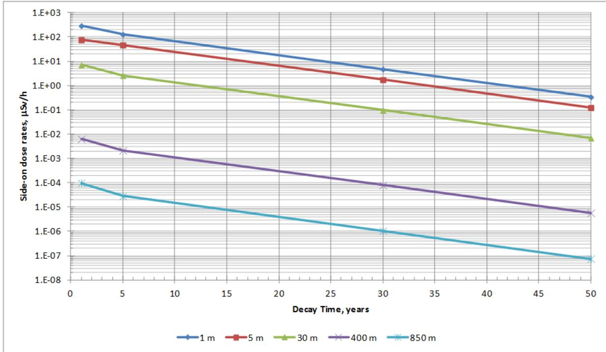
**Figure 5: Estimated Dose Rates from a DSM Containing Retube Components from Unit 1/2**
