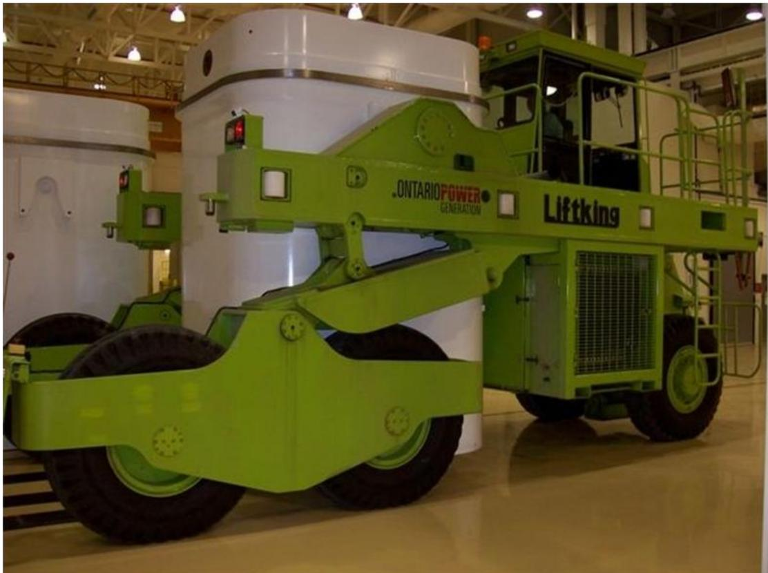
**Figure 10: Liftking DSC Transporter**
