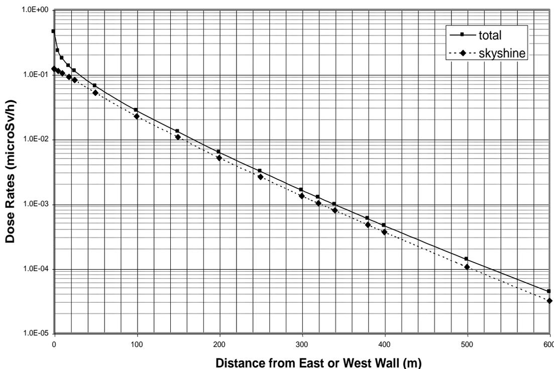
**Figure 14: Calculated Dose Rates from Phase II DSC Storage Buildings – East/West Walls**
